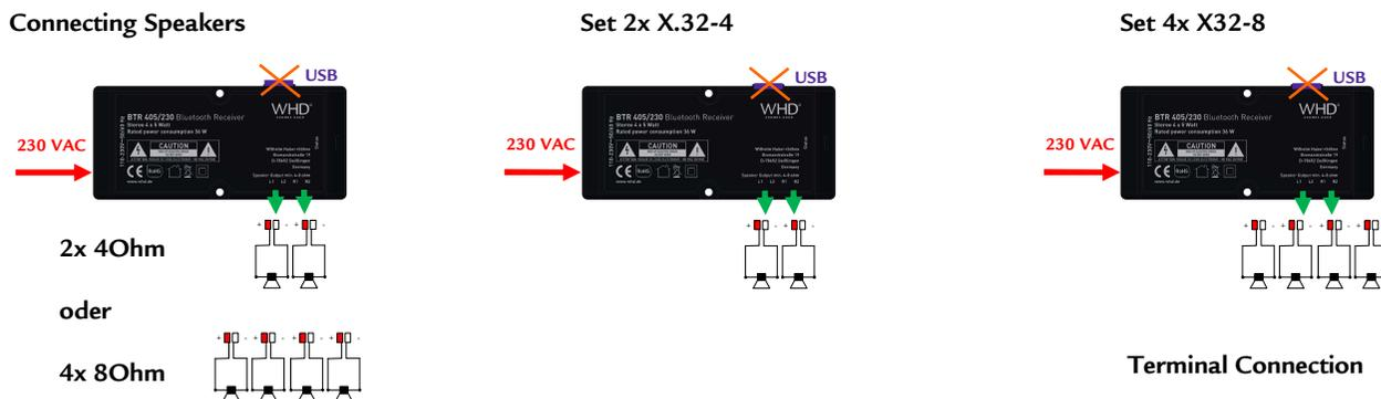
! USB connection is not active. Do not connect any USB device.
