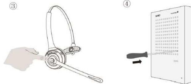
**Step 5.** Adjust the volume of the devices with a mini Phillips screwdriver when necessary.
