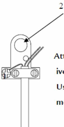
Attention! For safety reason it is compulsory to wind some of the ivory steel wire around screw (1) and tighten the screw.
